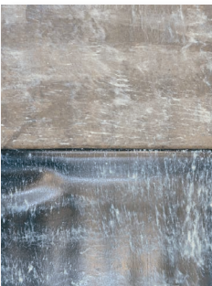
Firestone's Single-Ply LVOC Adhesive; Flash-off time 15 mins. 20 °F
