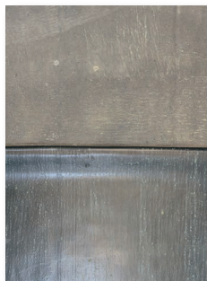
Competitor's Single-Ply LVOC Adhesive; Flash-off time 23 mins. 20 °F
